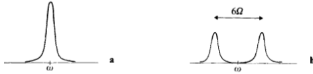
Figure 5: Split of resonance frequencies(degenerate)
