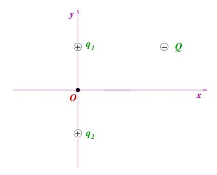
Positive charges  $q_1=3~\mu C$  and  $q_2=5~\mu C$  are placed along the y-axis at y=2.0 m and y=-2.0 m, respectively. A negative charge  $Q=-4~\mu C$  is placed at x=4.0 m, y=2.0 m.
