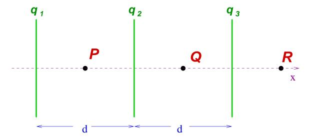
Three large parallel sheets have charges  $q_1=+2~\mu C,~q_2=+5~\mu C,$  and  $q_3=-7~\mu C.$  Each sheet has area  $A=1.5~m^2.$  Adjacent sheets are a distance d=4 cm from each other.
